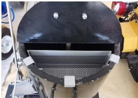
Paint Tank & Filter
