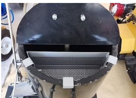
Paint Tank & Filter
