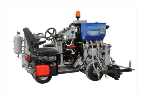
Features gasoline engine, hydraulic drive and mixing system. Thermal oil heating ensures the stability of thermoplastic paint. Cruise control maintains consistent coating thickness, with a control system that switches between virtual and real lines. The independent dual wheels provide balance while allowing flexible turning and easy control. Capable of working with screeding, extrusion or convex line applications, and can simultaneously complete marking arrows and letters.
