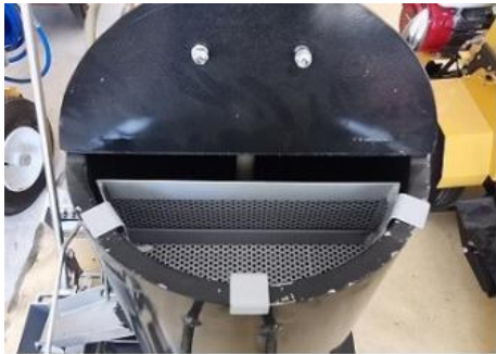
Paint Tank & Filter
