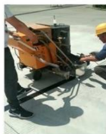
Thermoplastic road marking machine
